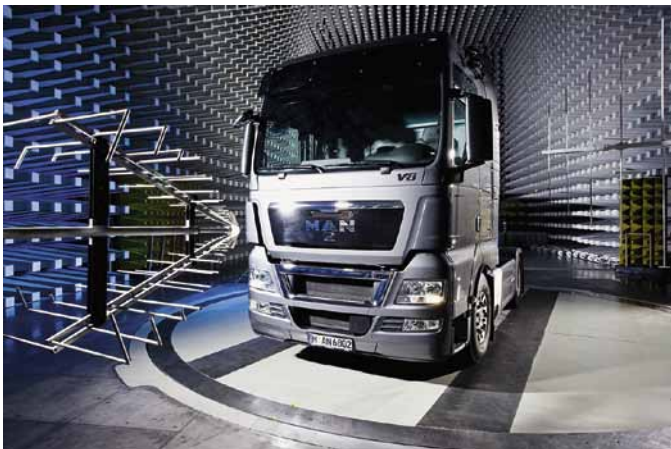
FIG 1 Radiated disturbance measurements with calibrated antennas.
