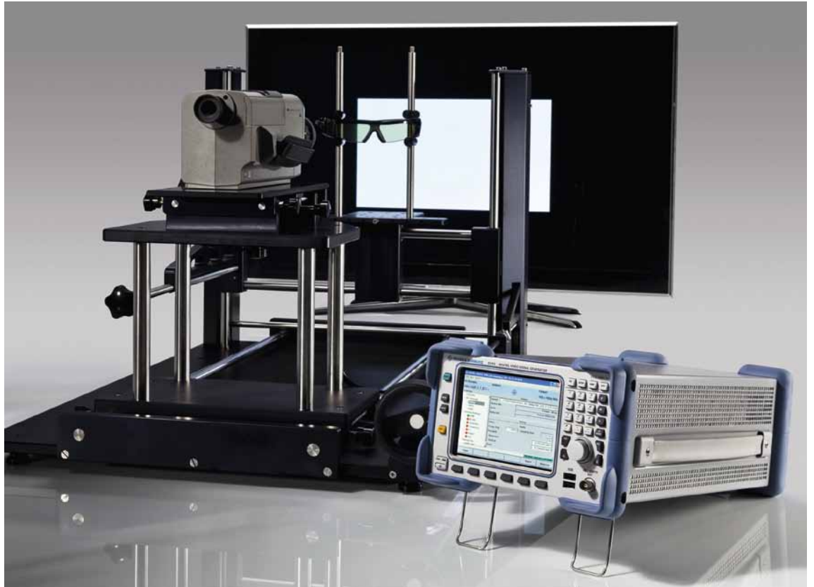
FIG 2 Typical test setup to measure the luminance of 3D TV sets (including a positioning system from Instrument Systems and a spectroradiometer from Konica Minolta).
