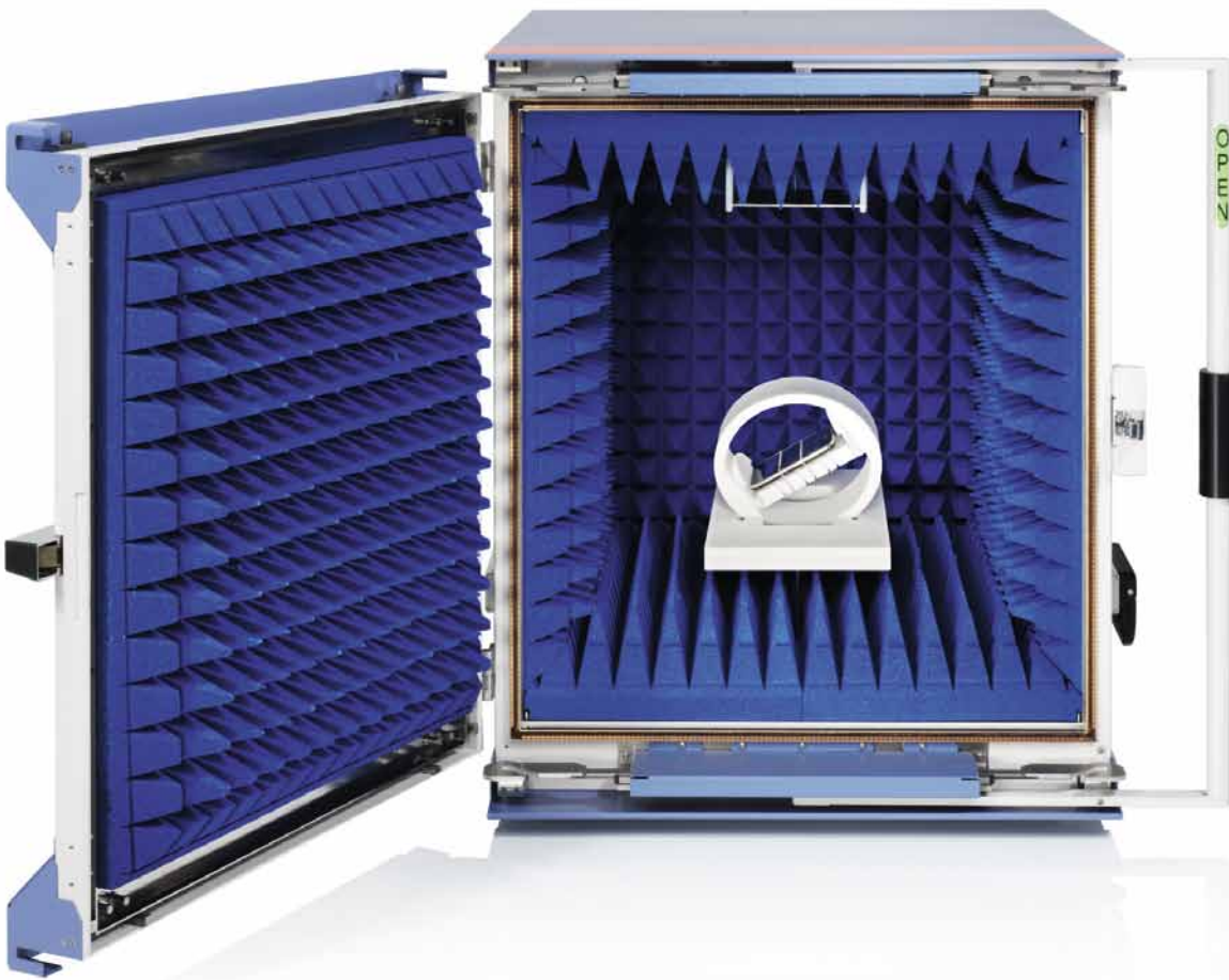
FIG 1 The R&S®DST200 RF diagnostic chamber with 3D positioner (R&S®DST-B150 option). It allows the user to position the EUT in any orientation relative to the test antenna with a turn of the wrist.
