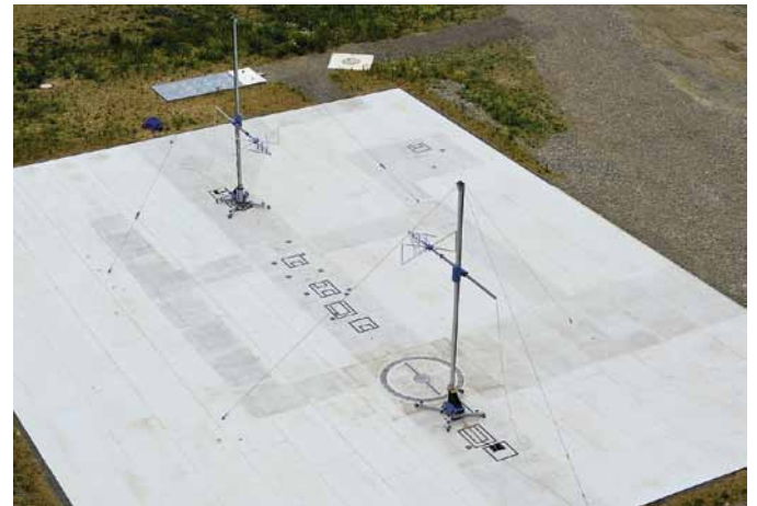
FIG 2 The open area antenna test site (20 m x 25 m) of Rohde&Schwarz Messgerätebau GmbH in Memmingen offers optimum conditions for high-precision antenna calibrations.
